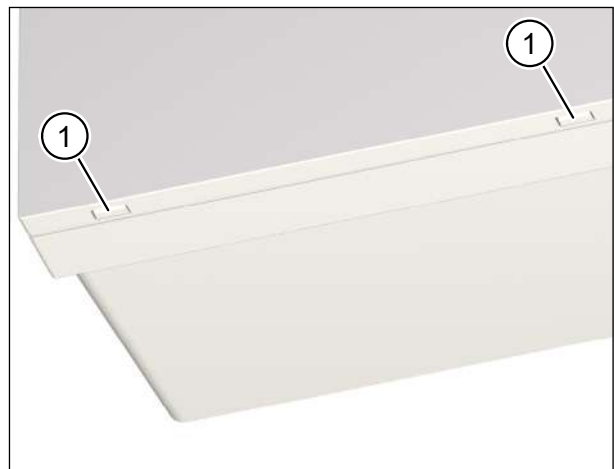
Fig. 22: Removing the unit cover from the ventilation unit
