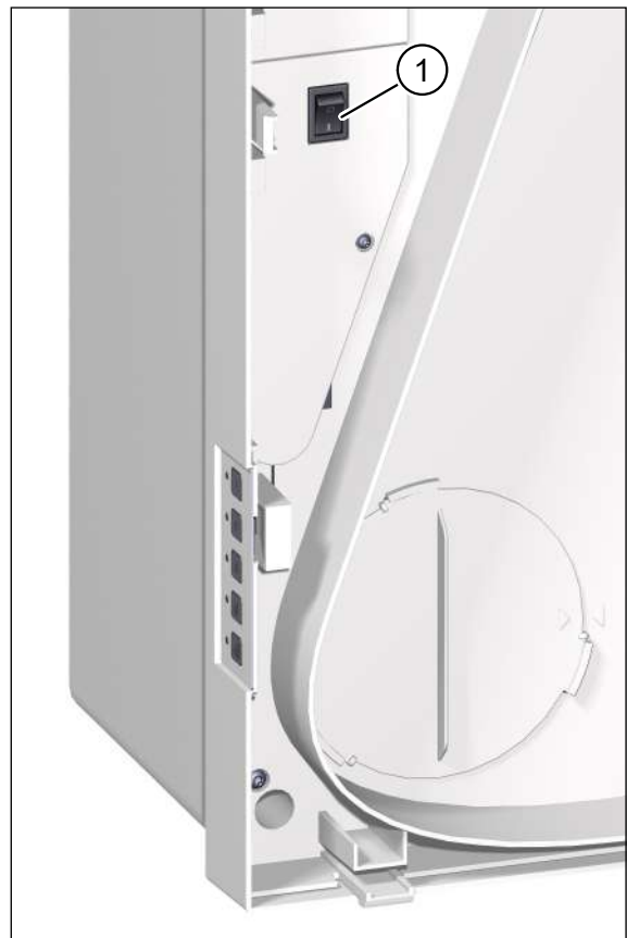
Fig. 4: Mains switch, visible when unit cover is removed
